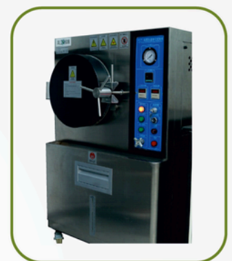
PRESSURE COOKER TEST (PCT)
